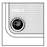
If your vehicle is equipped with outside heated mirrors, they can be defrosted by pressing the mirror button located near the fan control.
